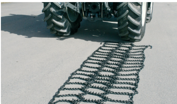
1. Put the chains behind the tyre with the fasteners against the tractor and the studs facing up.
