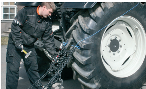
4. Drive forward one circuit, keep the chain narrow.
