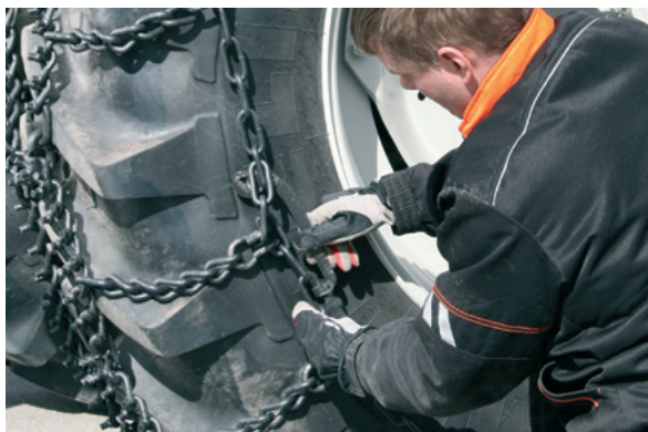
6. Fasten the chain with the fasteners inside first and then outside.
