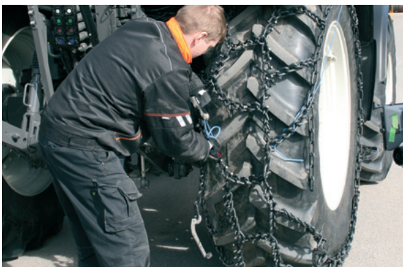
5. When the chain ends meet, connect the links by slanted gap couplings.
