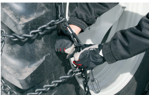
7. A good rule is that your hand should fit between the tyre and the chain. Do not tension too tight. Check tightness of the shackles.
