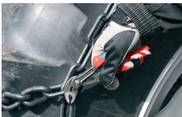
8. Check the tightening of the chain after a short test drive.
