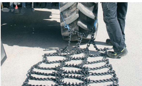
3. Put the rope on the top of the tyre.
