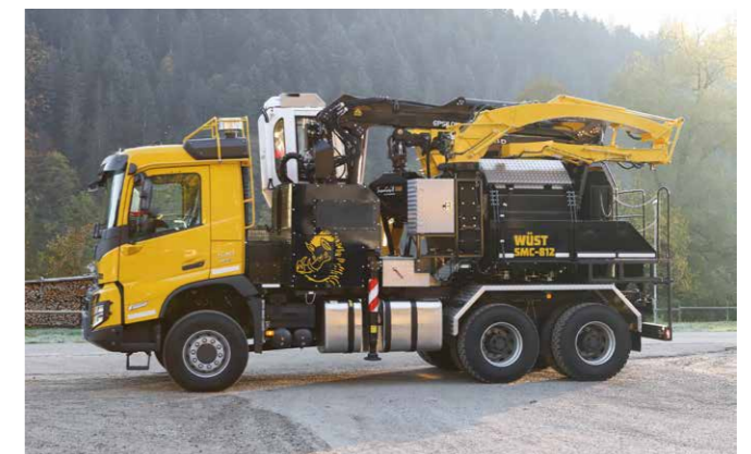
Wüst SMC-812 CCR (crane cab, infeed on the right) accelerator in center
