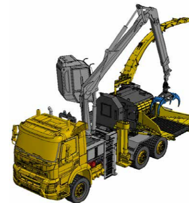
Wüst SMC-812 CCL (crane cab, infeed on the left) accelerator at the back
