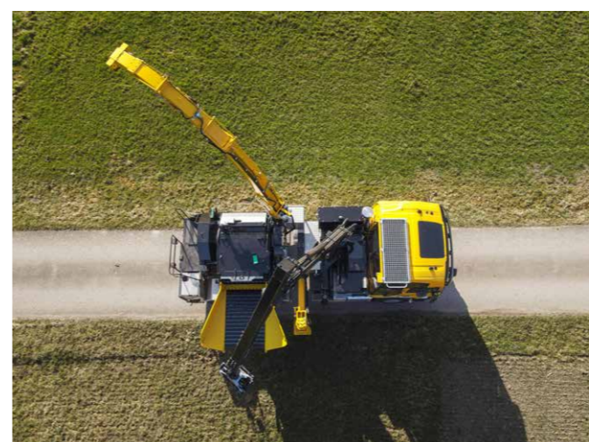
Volvo FMX, 540 PS with SMC-812 TCR, hydraulically driven accelerator, centrally arranged ejector spout
