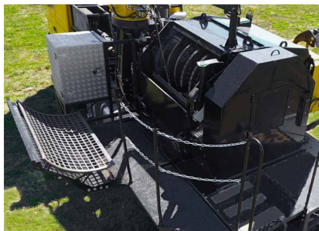
Maintenance platform with hydraulic folding and toolbox
