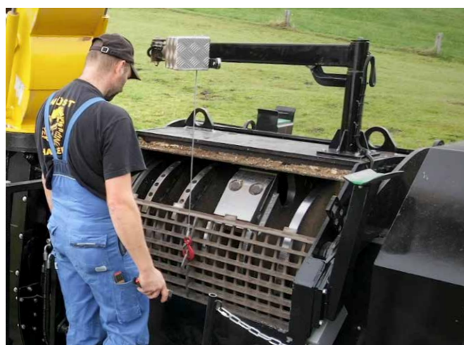
Electrical sieve crane above the rotor
