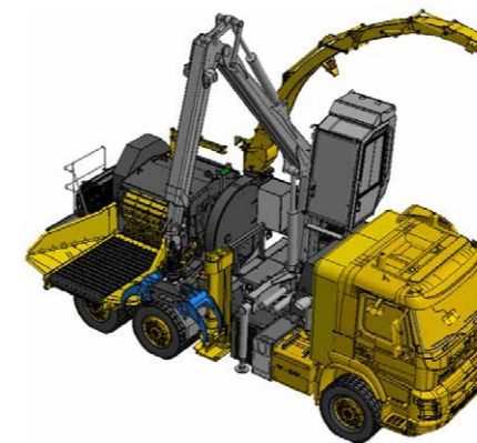
Wüst SMC-812 CCR (crane cab, infeed on the right) accelerator in center
