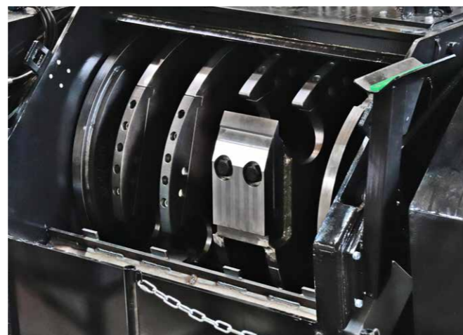
Rotor with a 200 mm cutter system, fitted with a depth limiter for variable cutting lengths of 15–45 mm.
