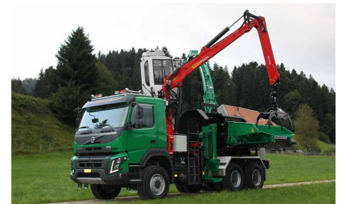
Wüst SMC-812 CCL (crane cab, infeed on the left) accelerator at the back
