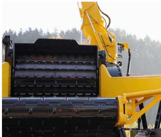
Upper infeed roll with interchangeable blades
