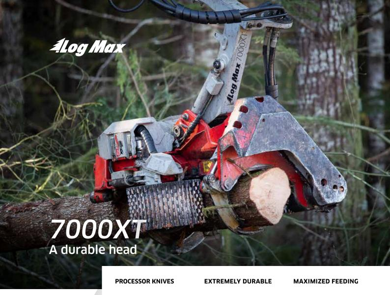
There are two different processor knives to choose from. A welded and a cast one.
